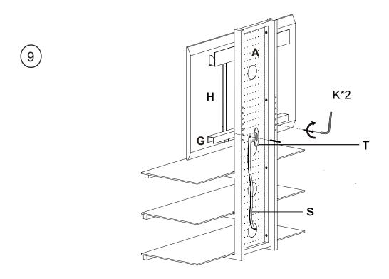
9-Attach holder (G) to bracket (H), fix holder (G) and wall strap(S) to panel (A) with washer(T) and screws (K).
